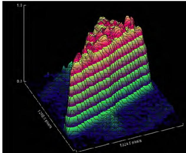
Figure 2. Sonoluminescence imaging indicating cavitation density and uniformity in the acoustic field of a 300 mm MegPie Transducer, energy  $2.9 \text{ W/cm}^2$  at 925 kHz. Each color cycle = 10%.
