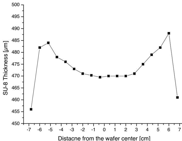
Figure 3. SU-8 coating uniformity over 150 mm diameter Si wafer.
