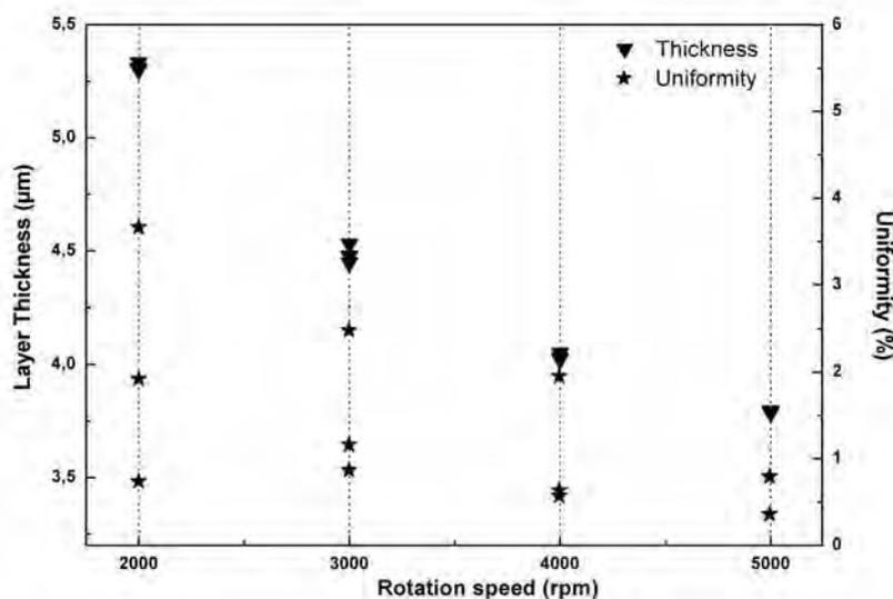
Figure 6. SINR™ layers thickness and thickness uniformity vs. rotation speed.
