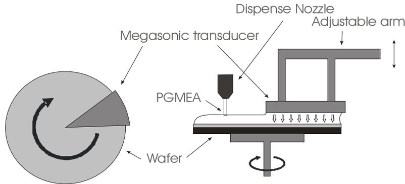
Figure 1. Horizontal spinner chuck system with fluid delivery and MegPie® transducer.
