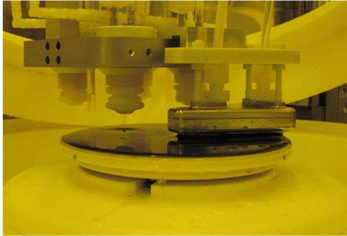
Figure 4. 150 mm single wafer megasonic-enhanced development system. Horizontal position of megasonic transducer and constant flow of developer are ensured.
