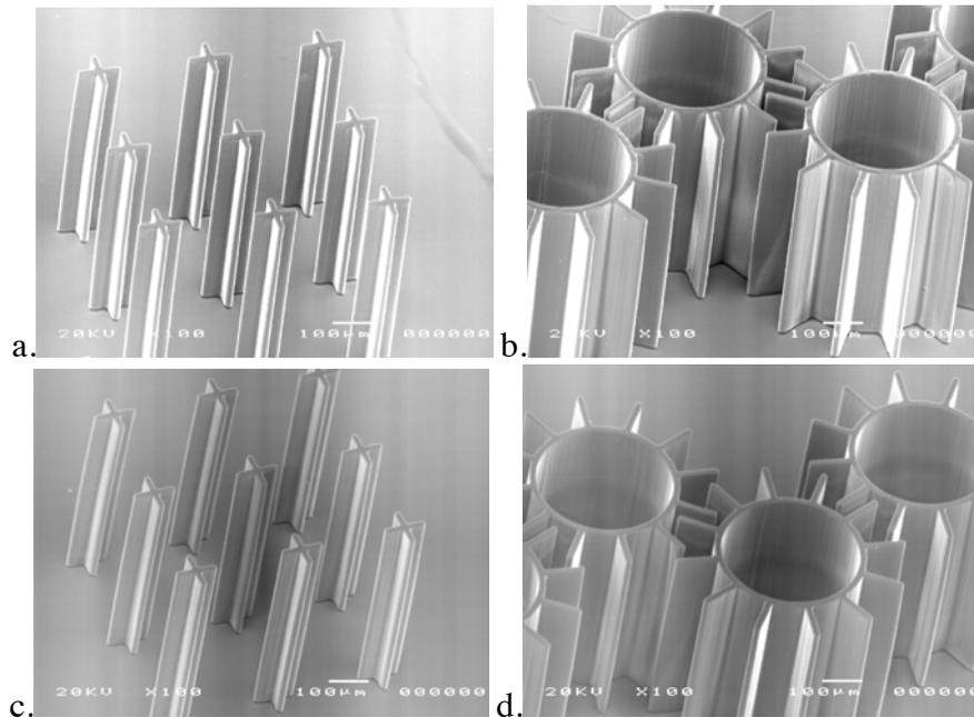
Figure 7. Free standing SU-8 structures:  $470\ \mu\text{m}$  high,  $20\ \mu\text{m}$  sidewall thickness, 1:23 aspect ratio. Structures a. and b. were developed in PGMEA bath for 240 min, structures c. and d. were processed with megasonic-enhanced development in 10 min.
