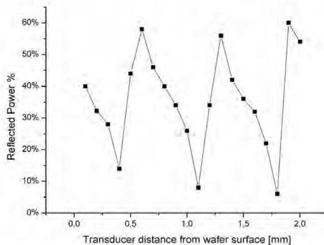
Figure 5. Reflected power as a function of the distance between megasonic transducer and the wafer surface.
