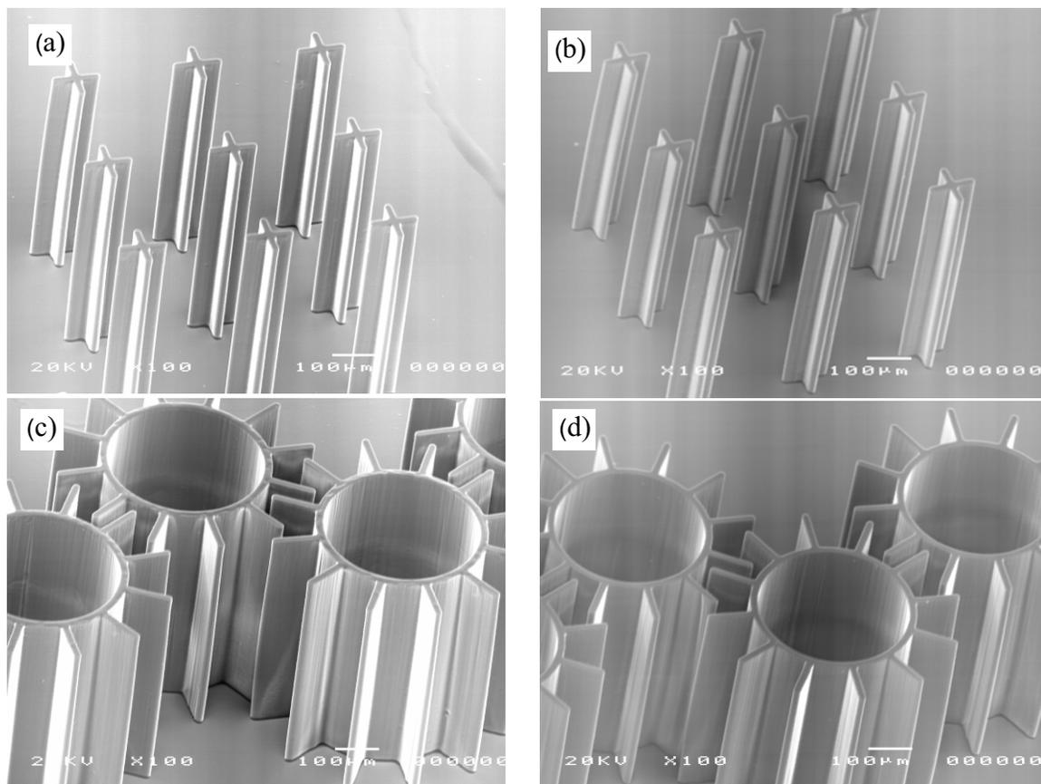
Figure 6. Free standing 470  $\mu\text{m}$  high SU-8 structures. Structures with sidewall thickness 20  $\mu\text{m}$ , aspect ratio 1:23. Structures on (a) and (c) were developed in PGMEA bath in 240 min, structures on (b) and (d) developed with single wafer megasonic-enhanced development in 10 min.
