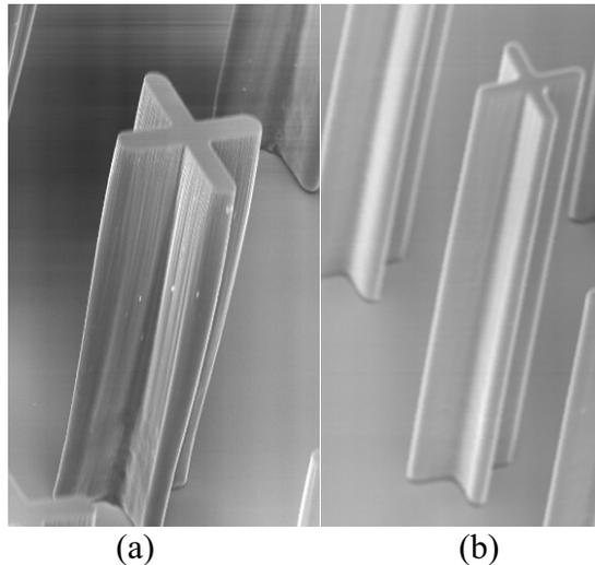
Figure 3. Structure profile (470  $\mu\text{m}$  high structures) depending on the exposure spectrum: structures exposed with 365 nm and 405 nm (a) show widening of top part of the structure; exposure with 405 nm only (b) leads to uniform line width on entire pattern height.
