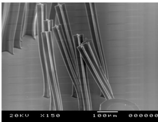
Figure 7. Distorted SU-8 structures, 470  $\mu\text{m}$  high with side wall thickness 10  $\mu\text{m}$ .
