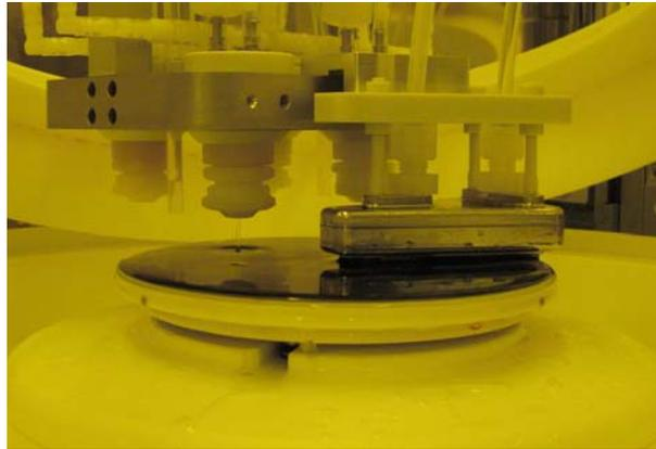
Figure 4. 150 mm single wafer megasonic-enhanced development system. Megasonic transducer integrated on dispense arm of EVG® 101 with adjustable horizontal position. Side view during development process. Dispense nozzle maintains constant flow of developer.
