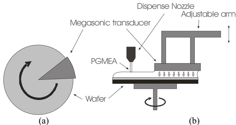
Figure 1. Schematic drawing showing the setup of the single wafer megasonic transducer: (a) view from top, and (b) cross section view.
