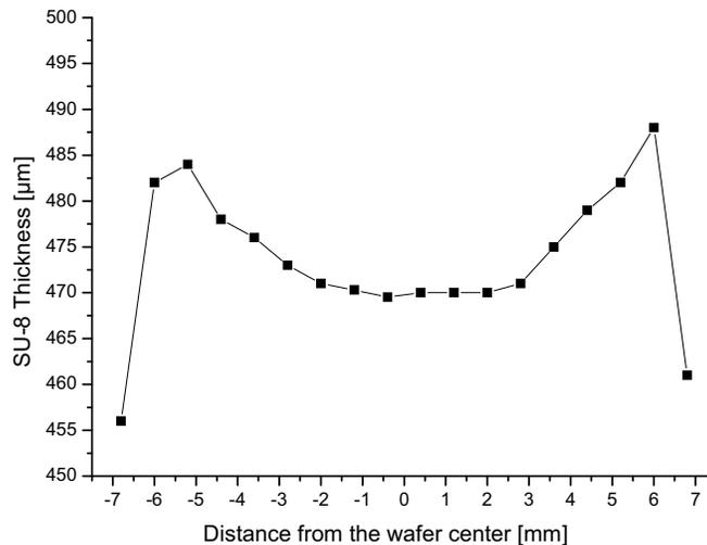
Figure 2. Coating uniformity of SU-8 over 150 mm diameter Si wafer.
