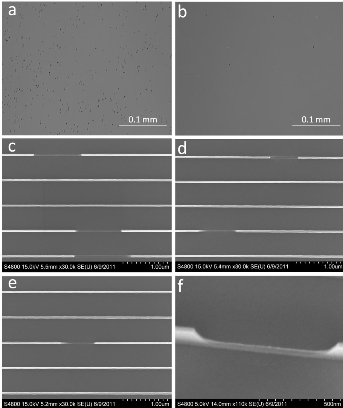
Figure 3. Microscope images of line breakages in Structures-I. (a,b) Optical microscope images at 200X and (c,d,e) FESEM images of line structures-I after 2 min irradiation to sound waves of power density 2.5 W/cm<sup>2</sup>. (f) FESEM image of a typical damage site at high magnification. (a,c,f) Damage induced in air saturated DI water. Damage induced in (c) 0.5 ppm CO<sub>2</sub>-DI water, (d) 412 ppm CO<sub>2</sub>-DI water and (e) 1035 ppm CO<sub>2</sub>-DI water.
