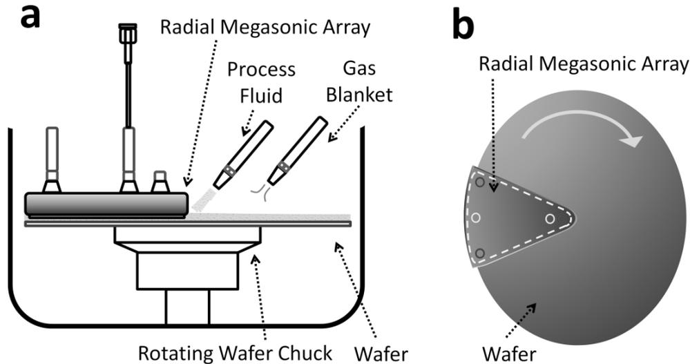
Figure 1. Schematic sketch of the single wafer spin-cleaning tool MegPie<sup>®</sup>. (a) Cross-sectional view and (b) top view.
