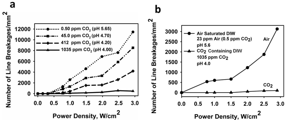
Figure 5. Plot of number density of line breakages in structures-I and structures-II as a function of megasonic power density and dissolved  $\text{CO}_2$  levels in DI water. (a) Structures-I and (b) structures-II.
