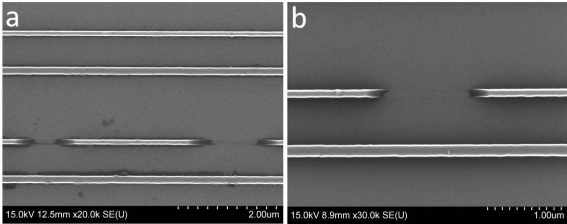
Figure 4. FESEM images of line breakages in Structures-II. FESEM images of line structures-II after 2 min irradiation to sound waves of power density  $1.5 \text{ W/cm}^2$  in (a) air saturated DI water and (b) 1035 ppm  $\text{CO}_2$ -DI water.
