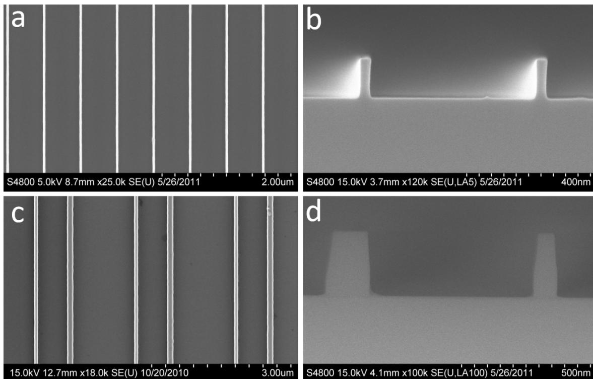
Figure 2. FESEM images of line structures-I and line structures-II. (a) Top view and (b) cross-sectional view of line structures-I. (c) Top view and (d) cross-sectional view of line structures-II.
