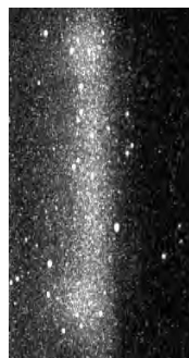
Figure 3: Sonoluminescence Measurements; a) test equipment; b) and c) photon imaging results for bottom and front transducers turned on.
