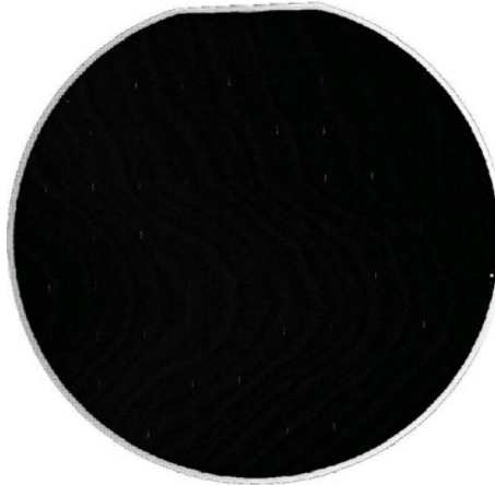
Fig. 7. Scanning Acoustic Microscope image of a 200 mm diameter CMOS wafer bonded to a blank Si wafer.
